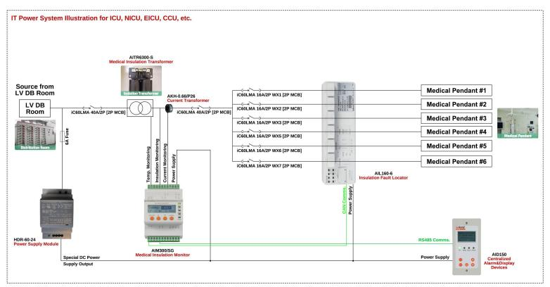
(1) Devices deployment in operating room for insulation monitoring [with fault location function]
