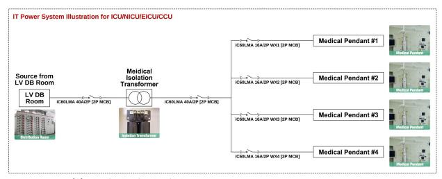
(2) ICU/EICU/NICU/CCU IT Power System Diagram Example
