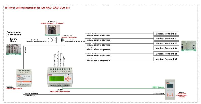
(1) Devices deployment in operating room for insulation monitoring [without fault location function]
