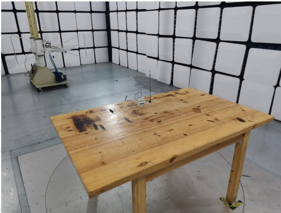
Photo of Radiation Emission Test
