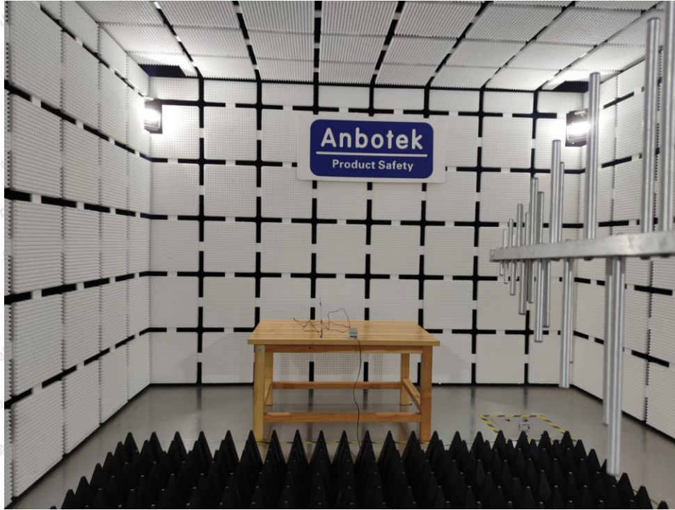
Photo of RF Field Strength Susceptibility Test
