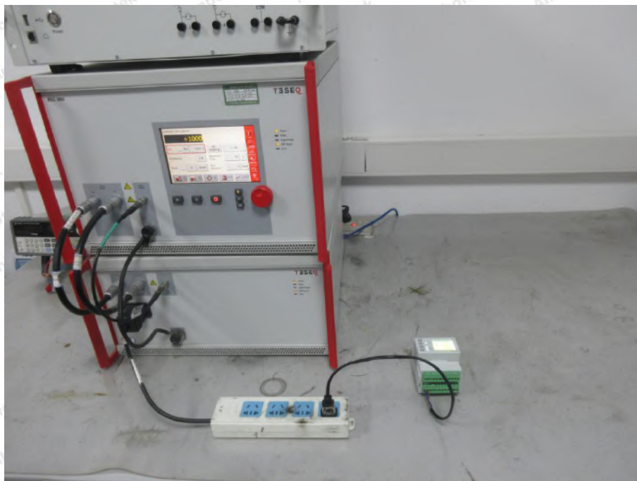
Photo of Surge Immunity Test
