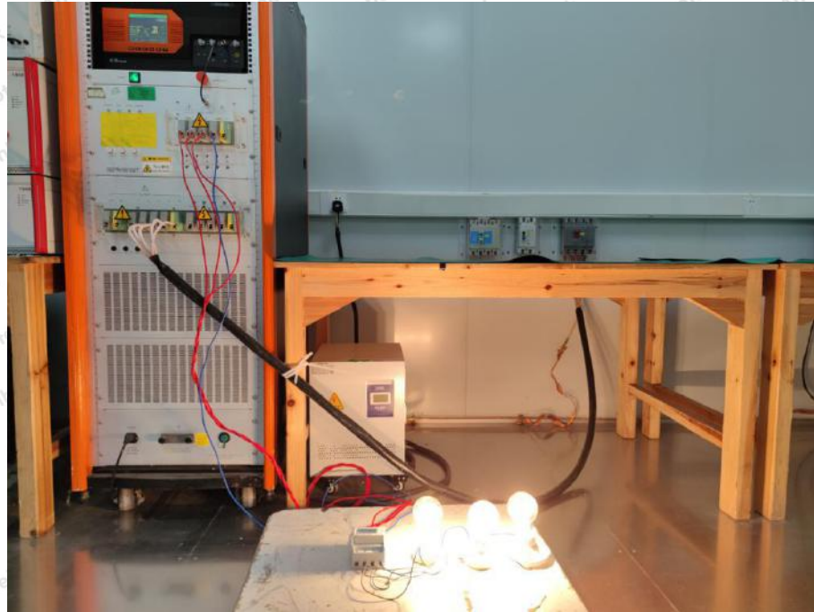
Photo of Electrical Fast Transient/Burst Immunity Test
