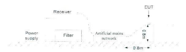
2. Test pic of conducted emission test
