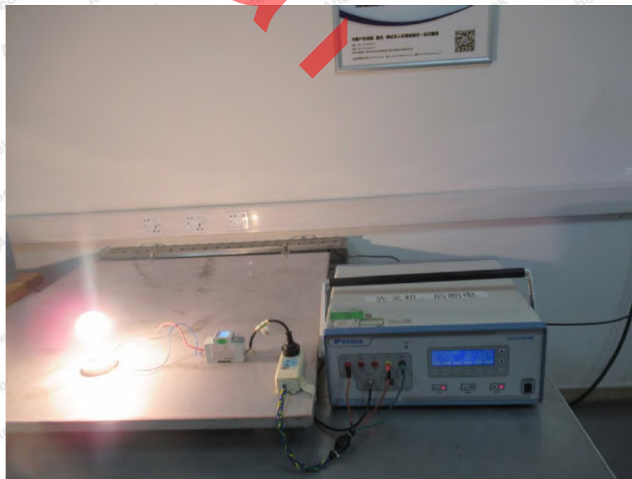
Photo of Electrical Fast Transient/Burst Immunity Test
