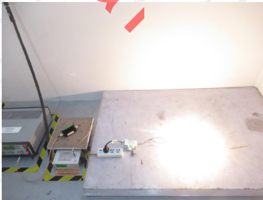
Photo of Injected currents susceptibility Test
