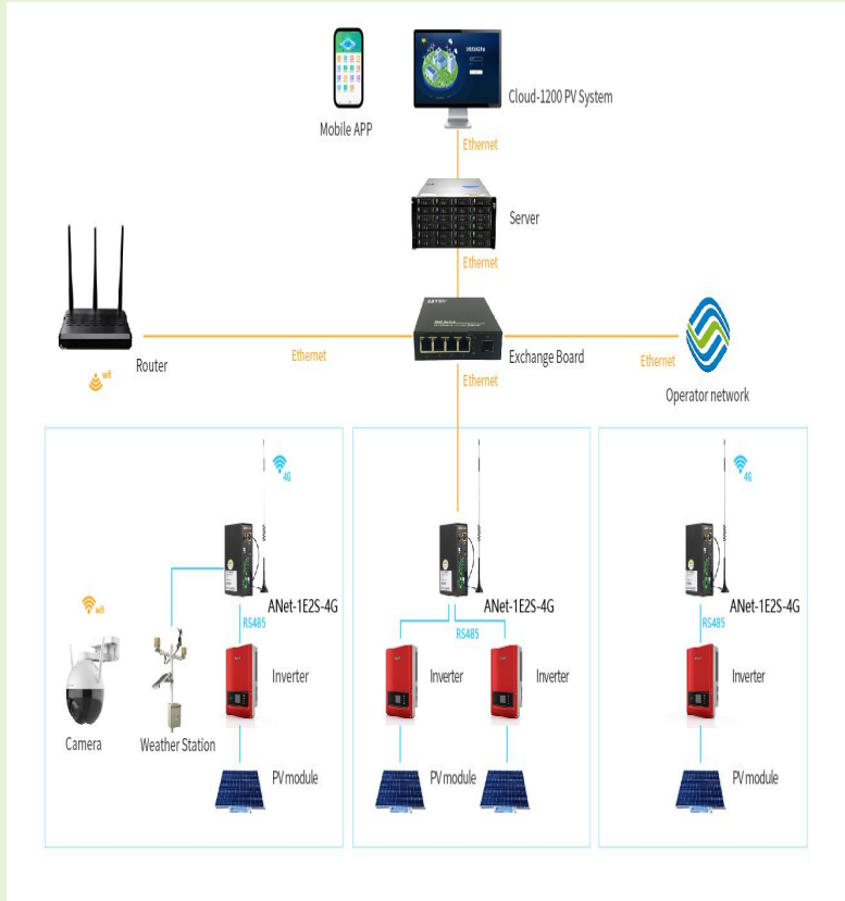
Acrel Cloud-1200 PV System Diagram
