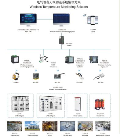
Wireless Temperature Monitoring Diagram
